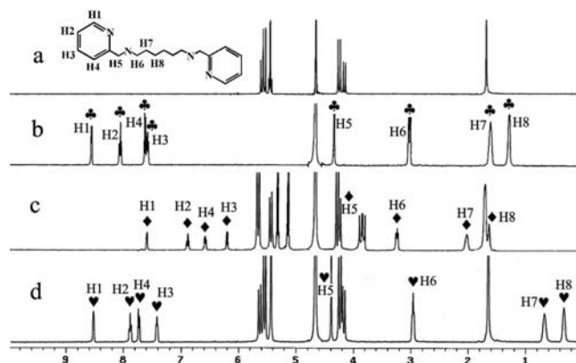
Figure 4. ^1\text{H} NMR spectra of (a) the host TMeQ[6] in \text{D}_2\text{O} , the N,N' -bis(2-pyridylmethyl)-1,6-hexanediamine in the (b) absence of TMeQ[6] and (c) presence of 2.0 equiv of the host TMeQ[6] in \text{D}_2\text{O} , and (d) complex 1 in \text{D}_2\text{O} .
